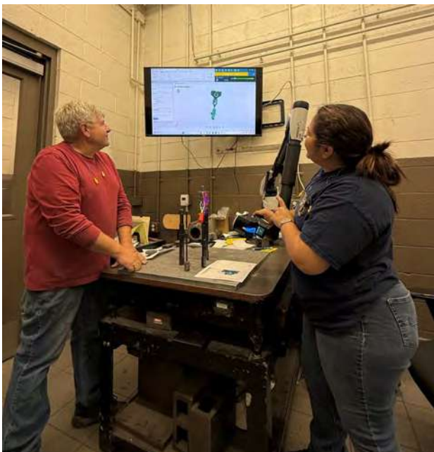
Randy Kadtko and Xenia Ponce scanning a part to reverse engineer.
